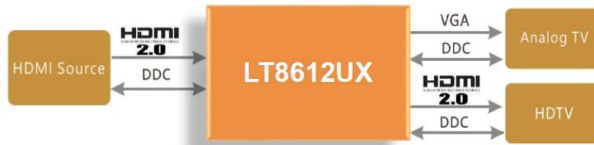
Figure 3.1 Application Diagram
